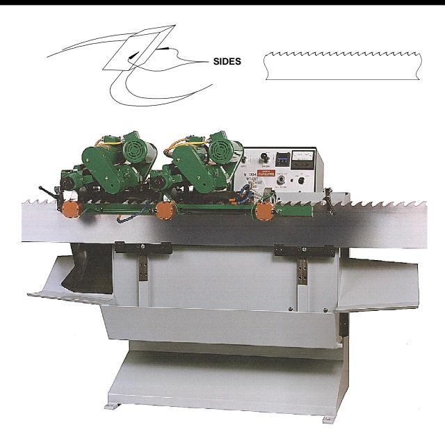
The W-1904 Quad quickly and accurately sharpens the sides of swaged or stellite® tipped band saws. Accurate side sharpening can increase saw performance and the W-1904 is our most accurate band saw sharpener.
