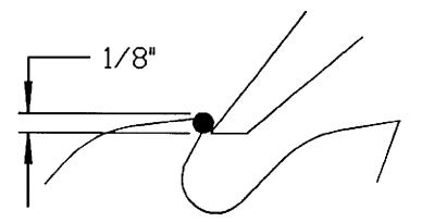
NOTE: The more accurate the height is set, less variation in Kerf will be experienced. If the tooth is placed higher a wider Kerf will occur. If lower, a narrower Kerf will occur.
