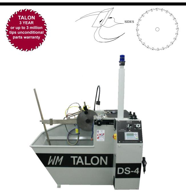
The DS-4 Dual Side Sharpener is accurate, productive, easy to operate and maintain. The DS-4 Dual Side grinder provides unbeatable accuracy which will improves saw performance greatly. Having the ability to single or multi-pass grind the DS-4 increases accuracy on thin plate saws by reducing grinding pressure.
